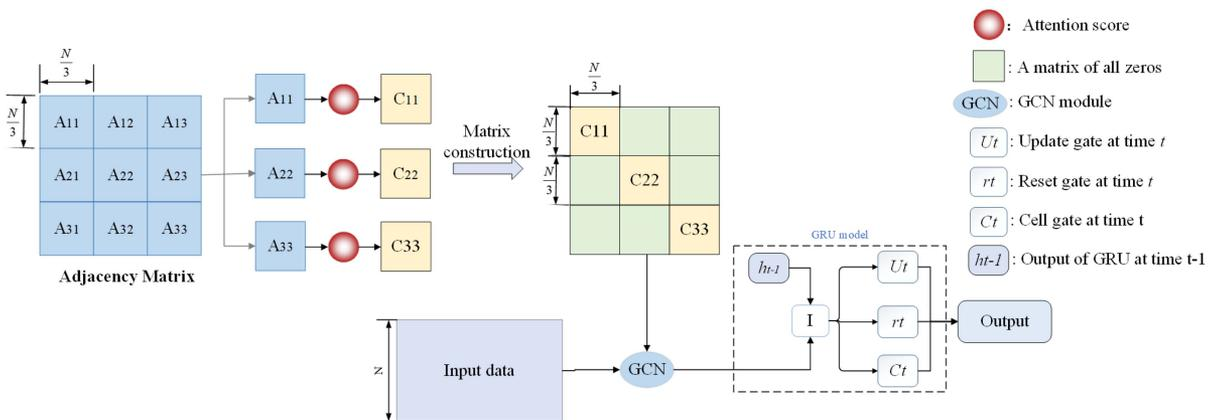
Fig. 5. Structure of GA-TGCN (when  $k=3$ ).
