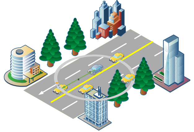
Fig. 2. Diagram of the relative position of the cooperative vehicle and the vehicle to be positioned
