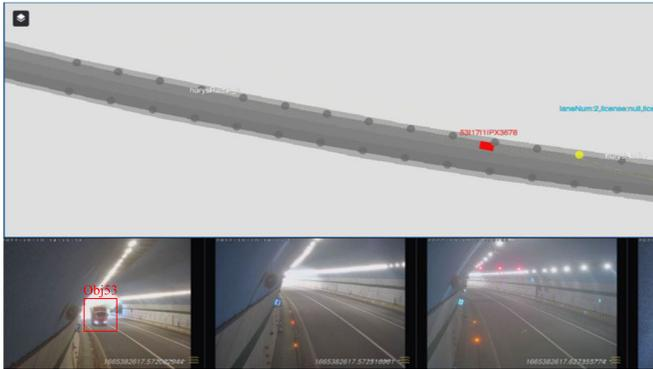
Fig. 6. Inaccurate radar measurements of large trucks.
